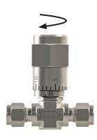
8. Move the micrometer barrel up under the handle so that the "zero" mark aligns with the bottom edge of the handle as shown. (The barrel may also be rotated to a position where measurements will be read from.) Then rotate the panel nut up against the barrel to temporarily hold it in place.
