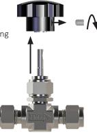
2. Use a wrench to remove the packing nut. (Make sure the packing springs are removed inside the packing nut.)
